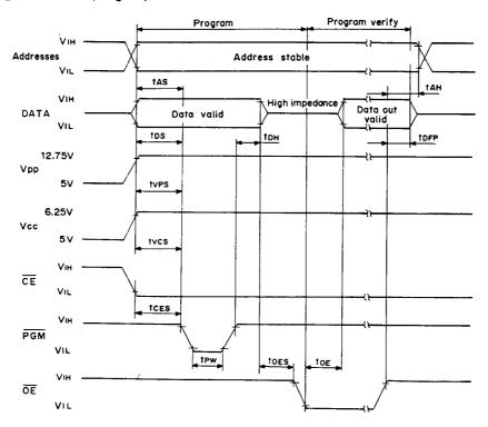
Note) When programming the CXK27C1001DQ a  $0.1\,\mu\text{F}$  capacitor is required access Vpp and GND to suppress switching noise caused by Vpp transient current.
