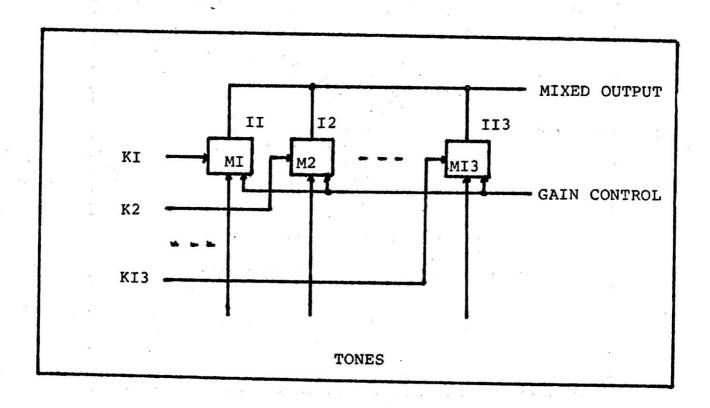
Each modulator produces an acoustic carrier (Tone), amplitude modulated from 0% to 100% by the corresponding k input voltage, around a constant d.c. level (offset current) equal to one half the maximum swing of each modulator output.
