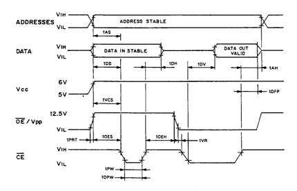
Note) When programming the CXK27C512DQ a 0.1 µF capacitor is required access  $\overline{\text{OE}}/\text{Vpp}$  and GND to suppress switching noise caused by Vpp transient current.
