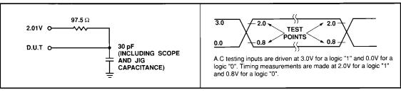
NOTE: 8. Provide adequate decoupling capacitance as close as possible to this device to achieve the published A.C. and D.C. parameters.
